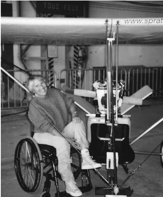
The Spratt 103 is easy for the physically challenged to access. No rudder pedals either. Below: the airframe is short at only 13 feet long. There are no elevator or rudders.
