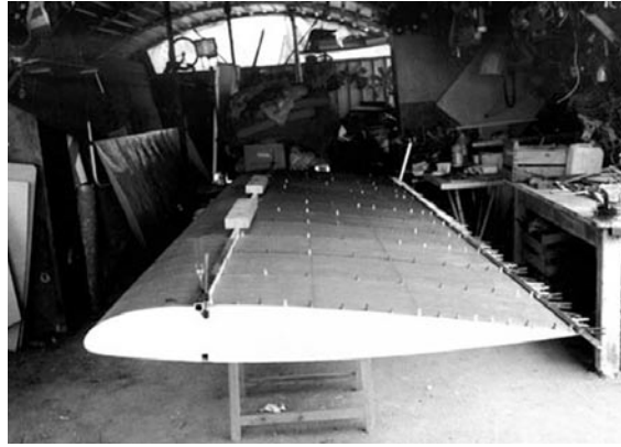
The ribs are attached to aluminum spars and fiberglass panels are glued on. The wings were tested to 4 g before deformation occurred.
